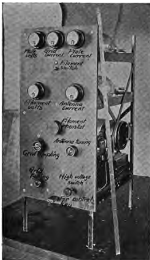
Fig. 65.—Continuous-wave transmitter using four Type P pliotrons; ammeters are supplied for plates and grids, and voltmeter for filament control.
